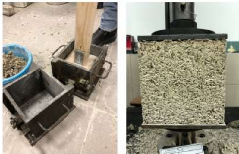
Figure 3. On the left: mold and hand rammer used for specimen forming. On the right: specimen prepared for the compressive strength test.
