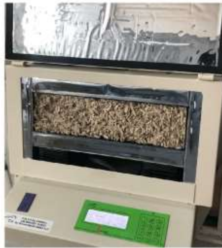
Figure 11. Thermal conductivity testing using the FOX 314 apparatus.
