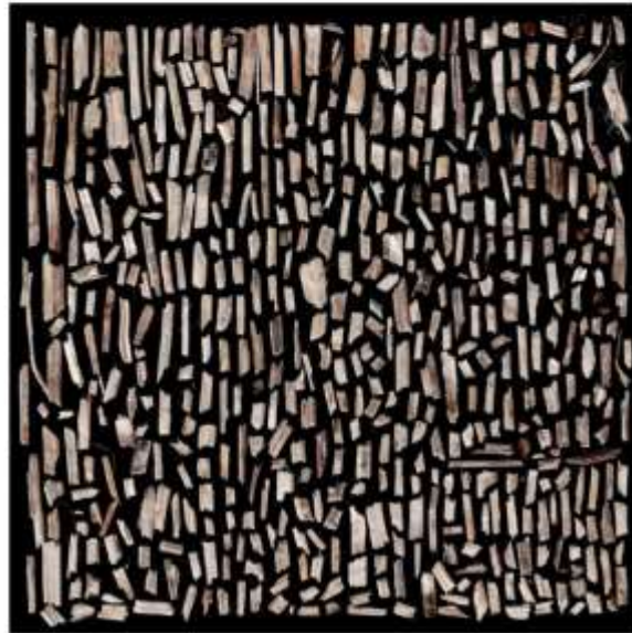
Figure 6. Sample scan of 3 g of hemp shives arranged on a 180 \times 180 mm surface.
