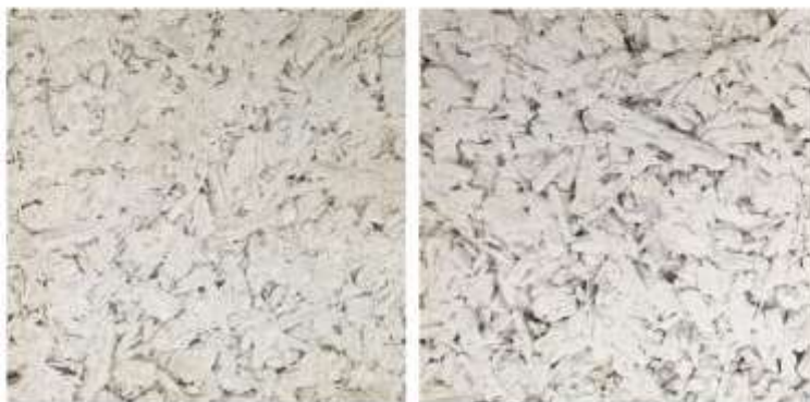
Fig. 7. The structure of hemp-lime composites with a hemp-lime ratio of 1:2 (right) and 1:1,5 (left).
