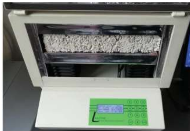
Fig. 2. Thermal conductivity test.
