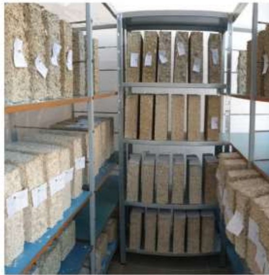
Figure 10. Samples from each series prepared for thermal conductivity testing.
