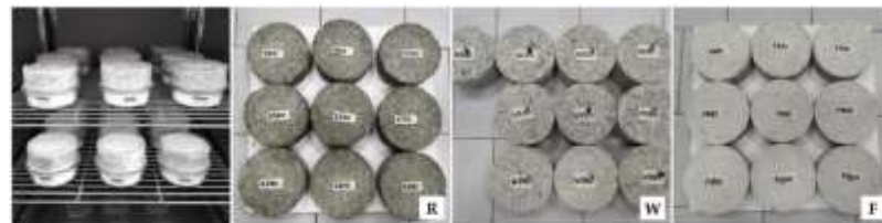
Figure 4. Sealed samples in climatic chamber and samples of all series prepared for water vapor permeability tests.
