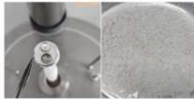
Figure 5. Hemp shiv sample in DSC crucible and example crushed sample of hemp-lime composite prepared for specific heat tests.
