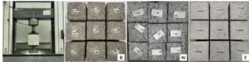
Figure 2. Instron 3382 machine and samples of all series prepared for compressive strength tests.
